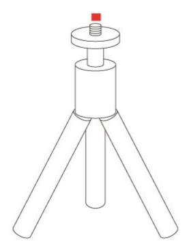
Tripods with 1/4 inch (M6×1) screws can be used with this product.
