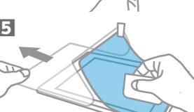
Once the position is decided, remove the remaining protective sheet while removing air bubbles using the film-attaching spatula and attach it on the liquid crystal screen.
