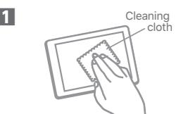
Please turn off the power supply of the main unit and wipe off the dirt on the screen cleanly with the attached cleaning cloth.
